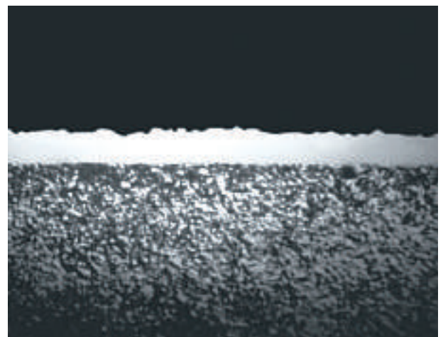
Cross-section of ATCoat coating
