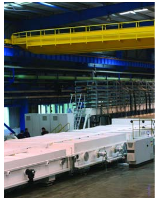
Glass coating unit for coating of glass with LowE- and Solar-Control-Coating
