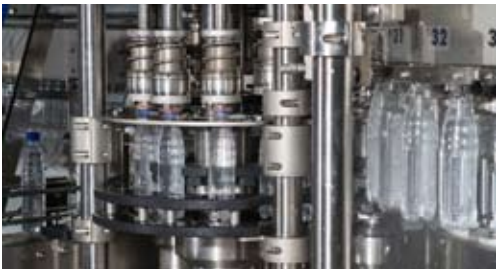
Capping Heads benefit significantly with Cerobear hybrid bearings which allow for an open cleanable design.
