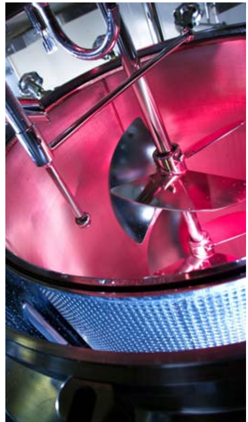
CEROBEAR rolling bearings are used in bio-m ® magnetic agitators of the sterile process engineering
