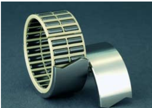
CEROBEAR Hybrid Engine Bearings feature silicon nitride rolling elements in a split PEEK cage and a two-piece hardened bearing shell. This advanced bearing technology significantly reduces friction losses and leads to an increased power output of up to 8%
