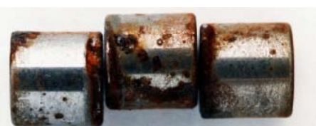
AISI 440 C ("corrosion resistant bearing steel")
